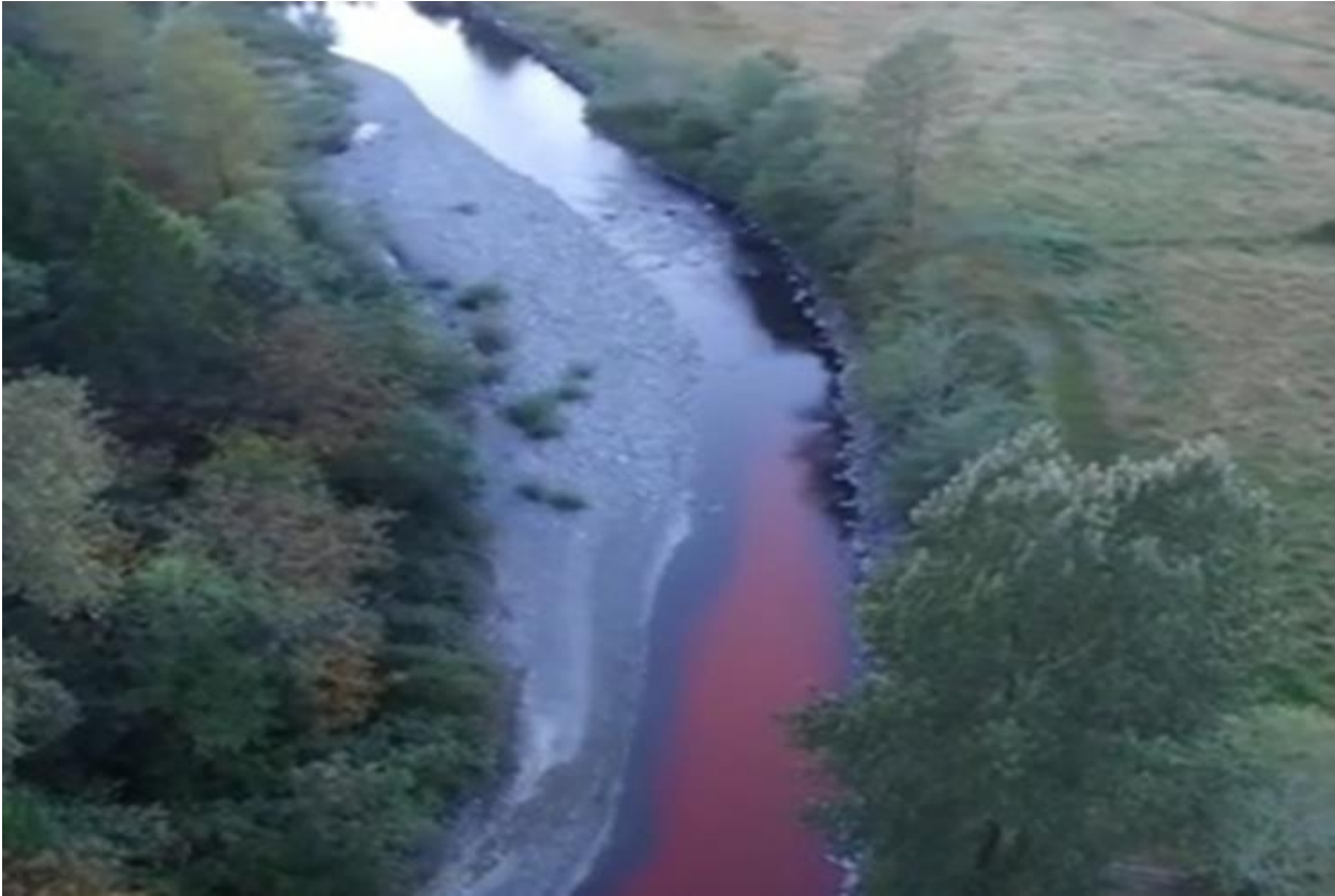
Figure 1. Advancing Dye Plume Simulating Chemical Plume in a River
