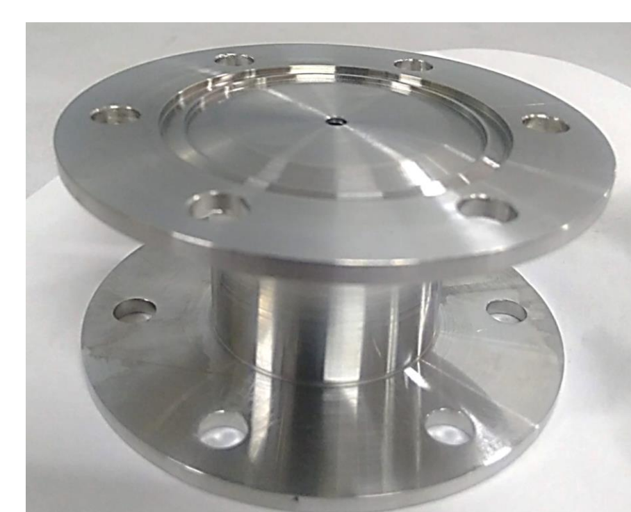
Figure 5. Fabricated hollow cathode isometric view
