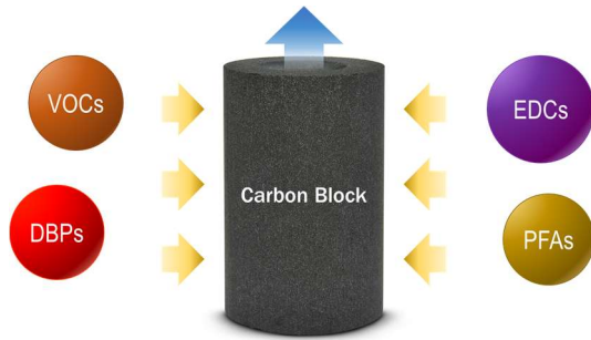
Figure 1. An example of an activated carbon block for the removal of organic contaminants in water.
