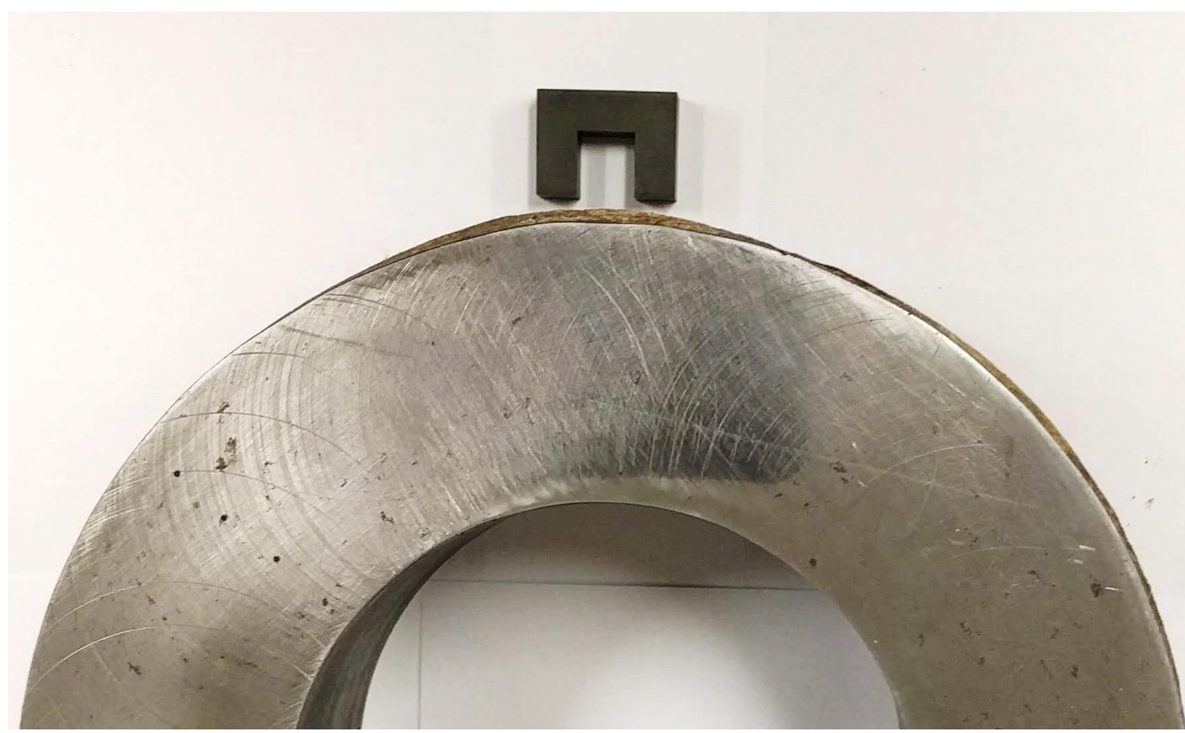
Figure 1. Cylindrical sample of HY-80 steel to be tested using MBN techniques. Radius of curvature: 50 mm.
