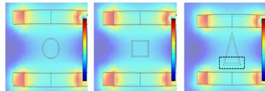
**Figure 4: Magnetic flux distribution across central pipe section for the circular, square and triangular cross-section flowmeters.**
