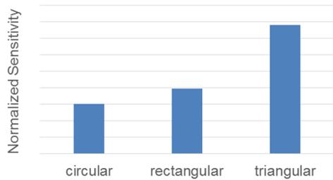
**Figure 5: Normalized sensitivity obtained from circular, rectangular and triangular cross section flowmeters.**
