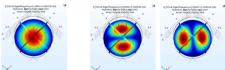
Fundamental mode (TM<sub>010</sub>), degenerate TM<sub>110</sub> modes, and TE<sub>011</sub> mode of single chamber.
