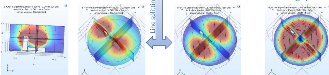
Additional line due to antenna, non-degenerate TM<sub>110</sub> modes, and TE<sub>011</sub> mode.
