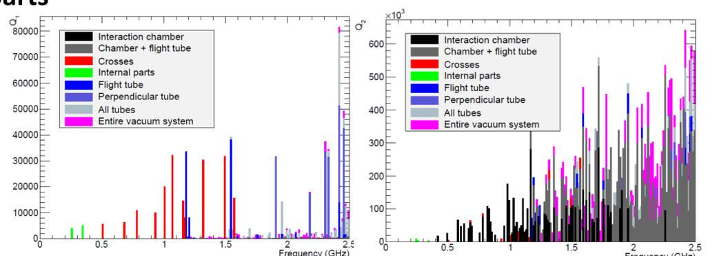
Eigenfrequencies weighted by Q-factors,  $Q_1 = \pi f_0 / \gamma$  and  $Q_2 = 2\pi f_0 W_t / P_d$ .
