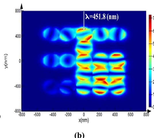
Fig. 7. (a) Transmission spectrum and (b) magnetic field ( $H_z$ ) distribution of the proposed XOR logic gate when a CW wave is launched to the input port A ( $A=1, B=0$ ).
