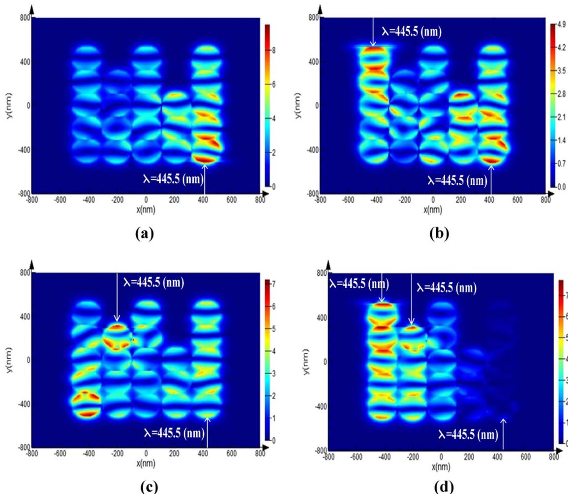
**Fig. 12.** Magnetic field ( $H_z$ ) distributions of the proposed NAND gate when (a) there is no signal at the input ports A and B, a CW wave is launched to the (b) input port A, (c) input port B, and (d) input ports A and B, simultaneously. In all states, a control signal is applied at control port.
