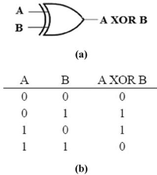
Fig. 4. (a) The circuit symbol and (b) the truth table of XOR logic gate.
