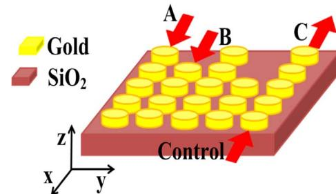
**Fig. 11.** Schematic view of the proposed NAND logic gate.
