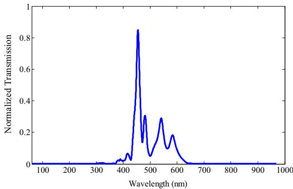
Fig. 6. Transmission spectrum of the structure of Fig. 5.
