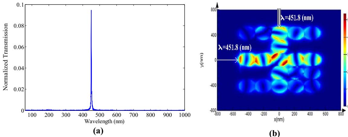
**Fig. 9.** (a) Transmission spectrum and (b) magnetic field ( $H_z$ ) distribution of the proposed XOR logic gate when a CW wave is launched to the input ports A and B simultaneously (A=1, B=1).
