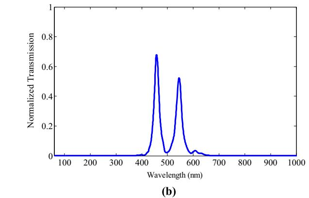
**Fig. 3.** (a) Schematic view of a non-periodic array of gold disk-shaped nanoparticles and (b) its transmission spectrum.
