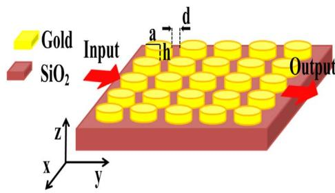
**Fig. 1.** Schematic view of a  $5 \times 5$  array of gold disk-shaped nanoparticles placed on  $\text{SiO}_2$  substrate.
