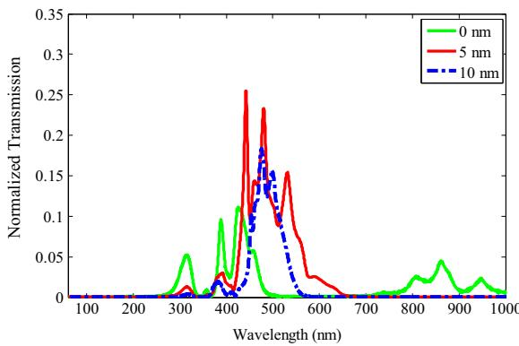
**Fig. 2.** Transmission spectra of the array structure of Fig. 1 with the inter-particle spacing of 0, 5, and 10 nm.
