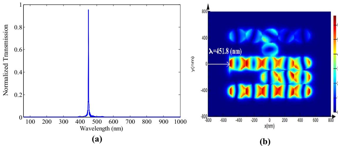
**Fig. 8.** (a) Transmission spectrum and (b) magnetic field ( $H_z$ ) distribution of the proposed XOR logic gate when a CW wave is launched to the input port B (A=0, B=1).
