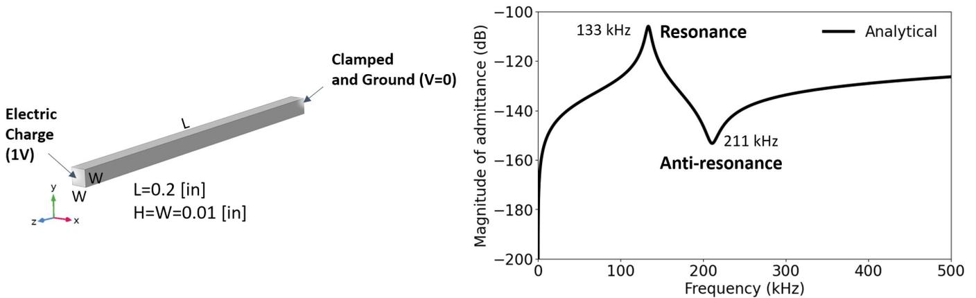
**Figure 1** : Admittance Spectrum of PZT Slender Bar
